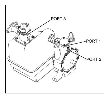
Figure 20 (12-20 kW) Gas Pressure Test point
